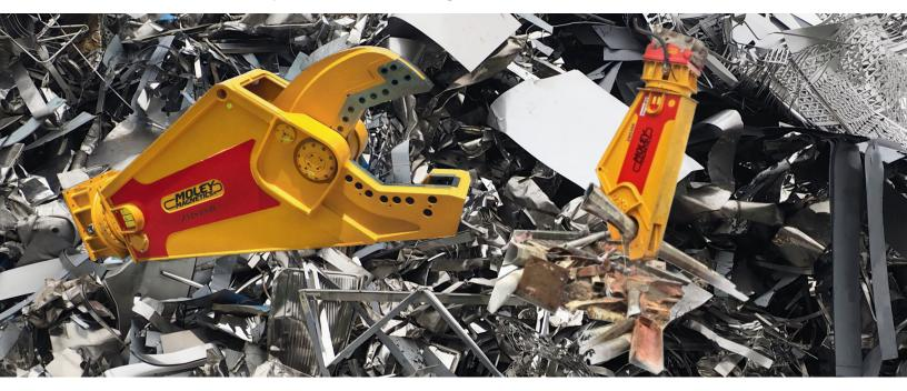
Moley Shears have four turn blades for maximum cutting life, 15% increased force, a strengthened cylinder with longer stroke, speed valve, and a super-reinforced HARDOX totally closed upper body that protects the clyinder and provents distortion
