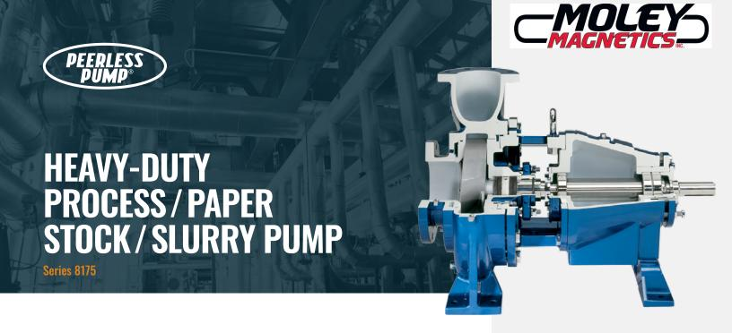
Manufactured for a wide range of flow and head requirements, the Peerless Pump 8175 Series process pump is engineered for lower operating costs. The back-pullout assembly can be replaced without removing the coupling and motor. The extra-thick casings and heavy-duty shafts and bearings are ideal for the toughest of services. The 8175 Series pump is interchangeable with competitors' pumps, and all 8175 Series power ends are backed by our three-year warranty.
