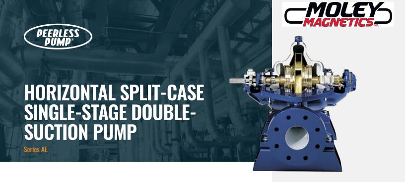
Using the latest technology, Peerless Pump engineered the AE Series pump to accommodate a variety of applications. The single-stage, double-suction, horizontal split-case pump comes in 42 different hydraulic configurations and 25 pump sizes. Discharge sizes range from two to ten inches. The AE has a wide selection of hydraulic performance envelopes, multiple mechanical configurations and several material options.
